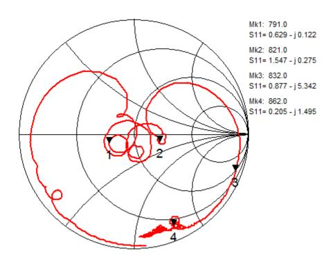
Fig.5 Impedance (Input)
