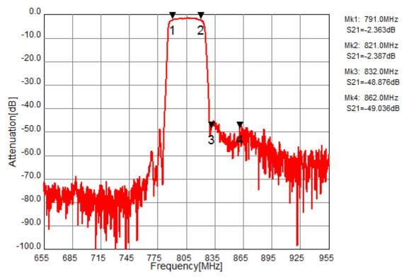
Fig.1 Pass-band Characteristics
